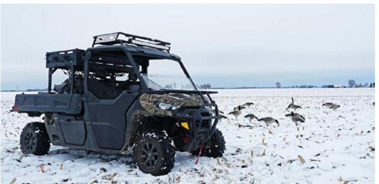
Specs: Engine: 82 hp/69 lb-ft, Rotax 976 cc, V-twin; Towing Capacity: 2,500 lb; Payload Capacity: 1,700 lb; Cargo Box Capacity: 1,000 lb; Wheelbase: 115.5 in.; Ground Clearance: 13 in.
